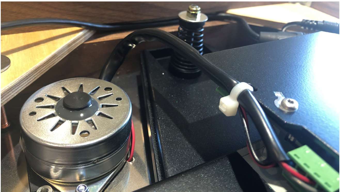
Figure 28 – dressing/containing the motor and sensor wires so as to avoid contact with the sub-chassis
