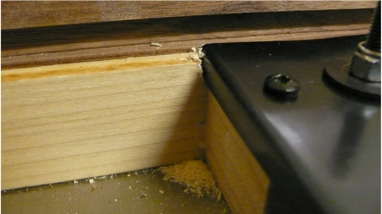
Figure 18 – Slotting the support rail either side of the blocks so as the cross-member can attach properly
