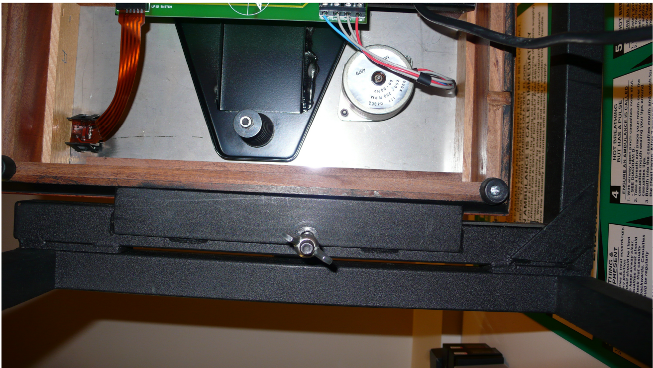
Figure 4 – A plinth in the jig sliding between the plinth supports when being clamped
