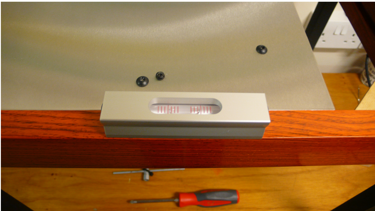
Figure 6 – Making sure that the plinth is level
