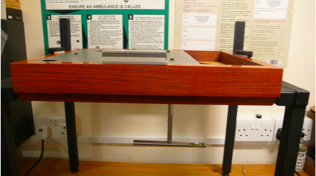
Figure 7 – Using the T-bar so that the spring hanger bolts are vertical
