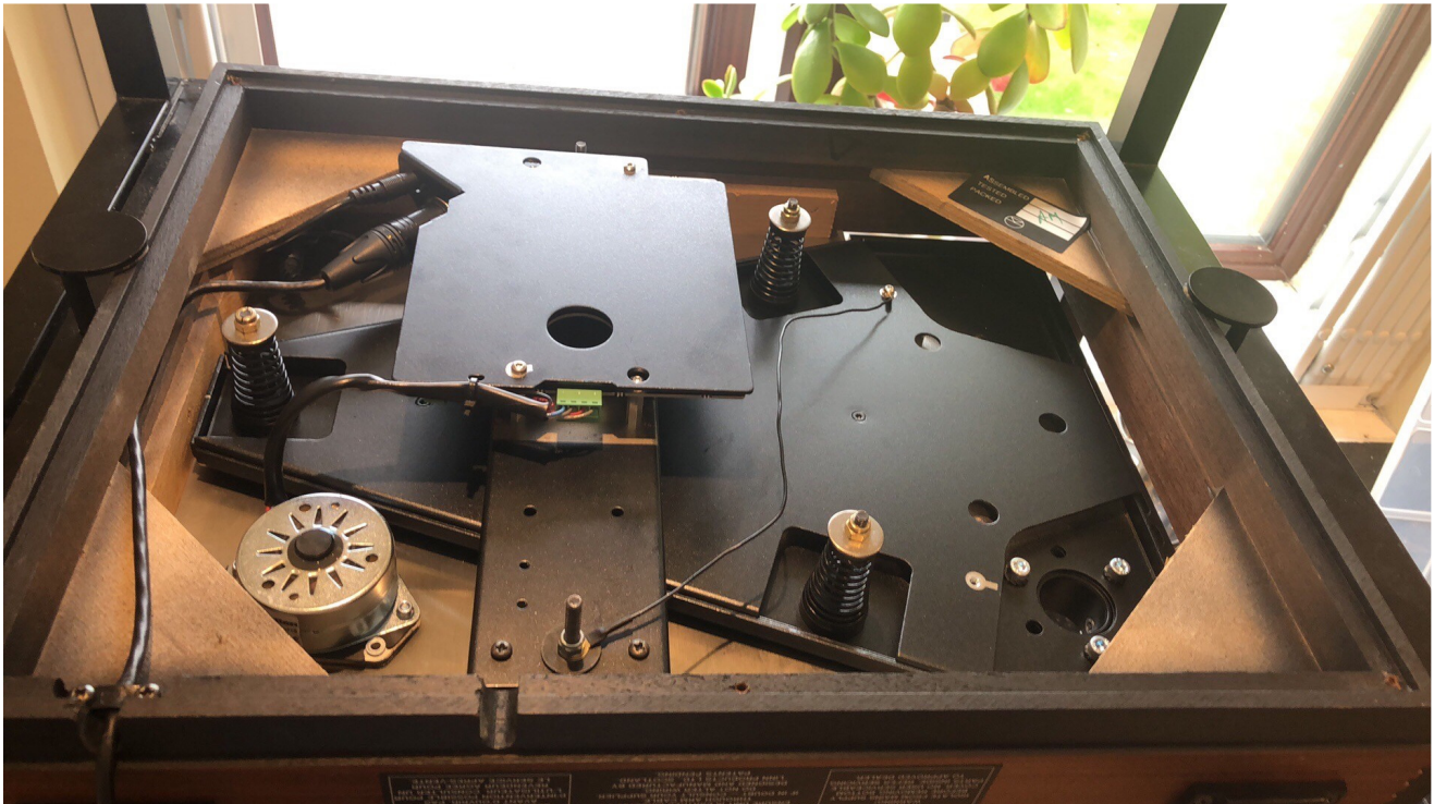
Figure 26 - The Lingo 4 installation is very different as seen here – Note orientation of the sub-chassis earth wire!
