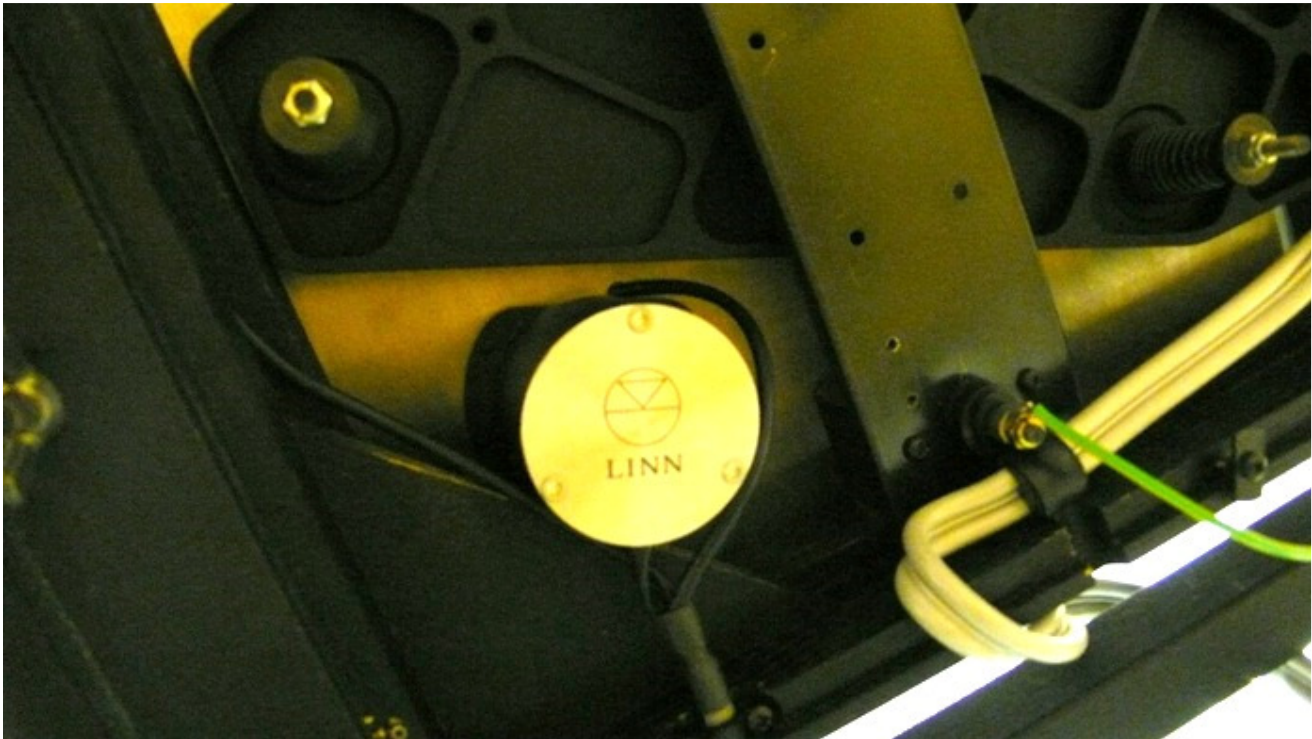
Figure 33 – Radikal speed sensor wires must be dressed round the motor to avoid contact with the Keel
