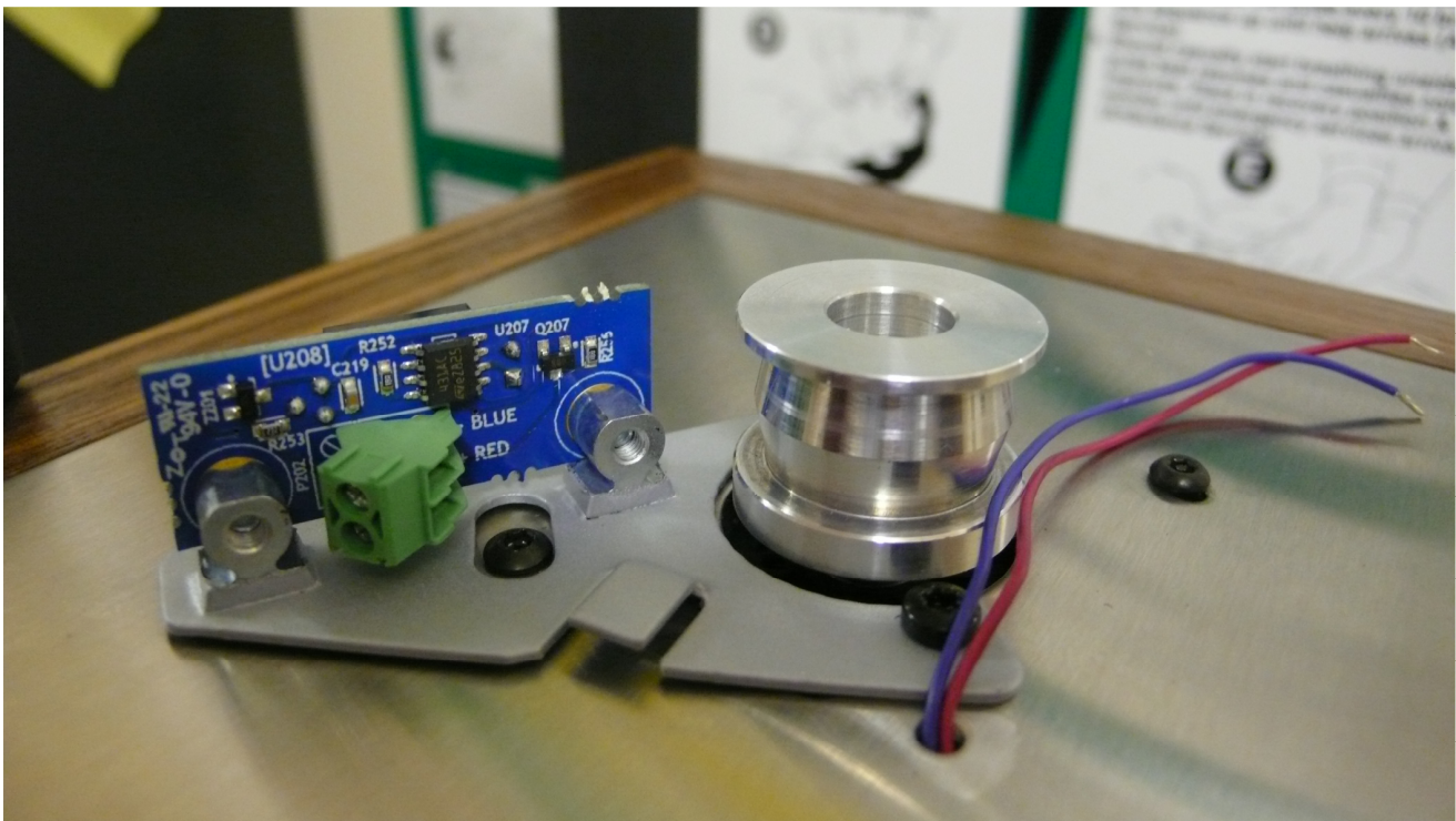
Figure 31 – Threading the wires for and the fitting of the Radikal speed sensor (same layout for the Lingo 4)
