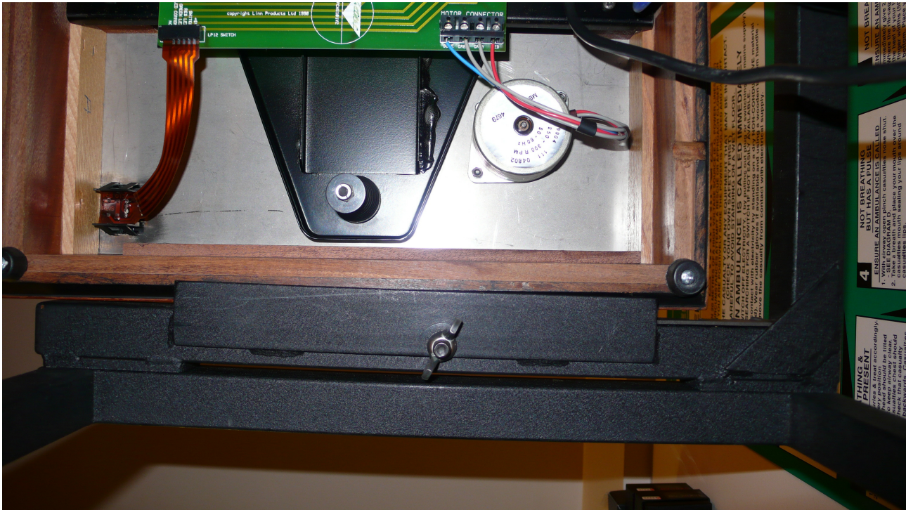
Figure 5 – Diagonal clamping of plinth in the jig giving support where before there was little/none
