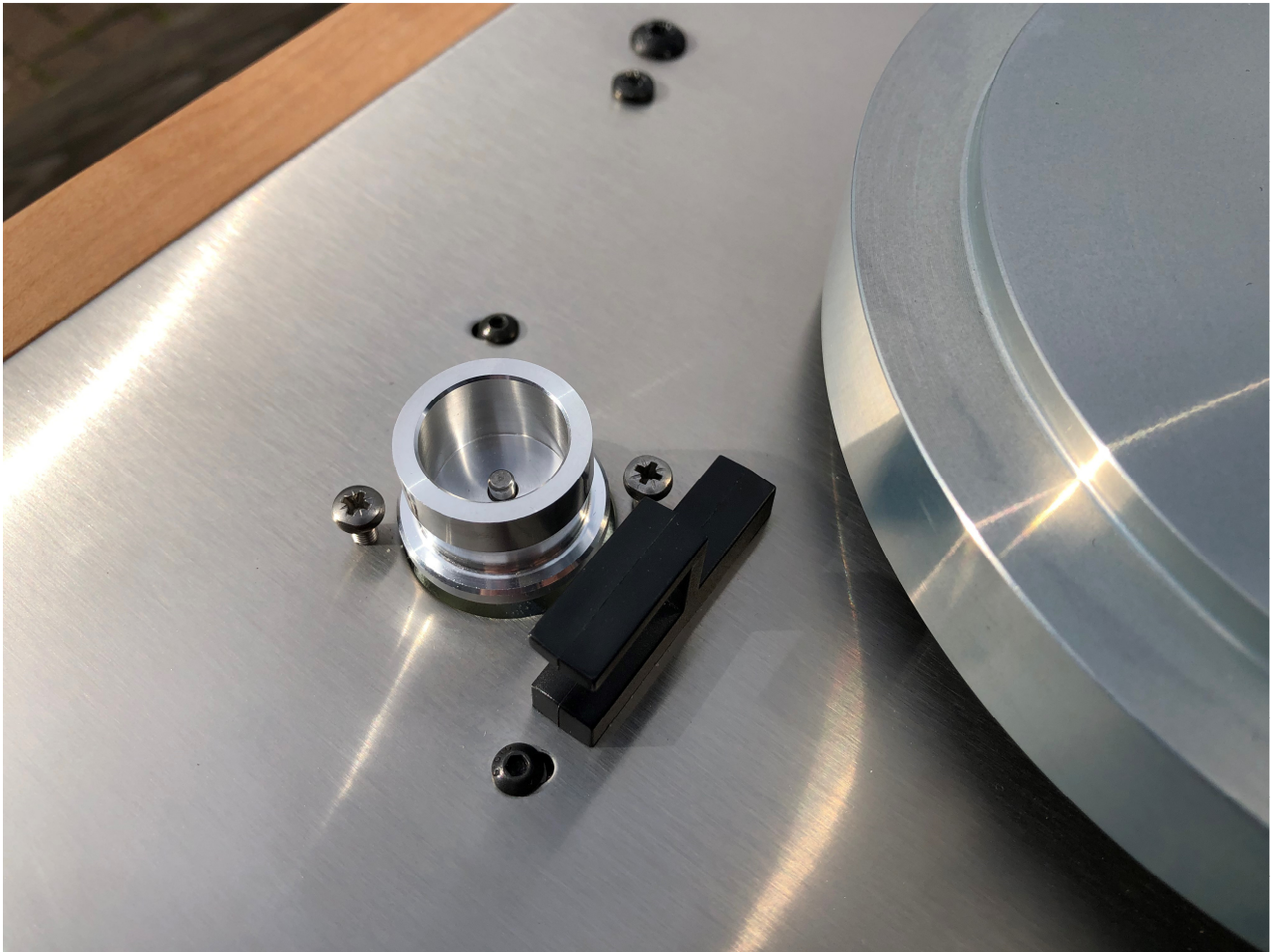
Figure 89 – shows the hexagonal motor mounting bolts and the silver Pozi speed adjustment screws
