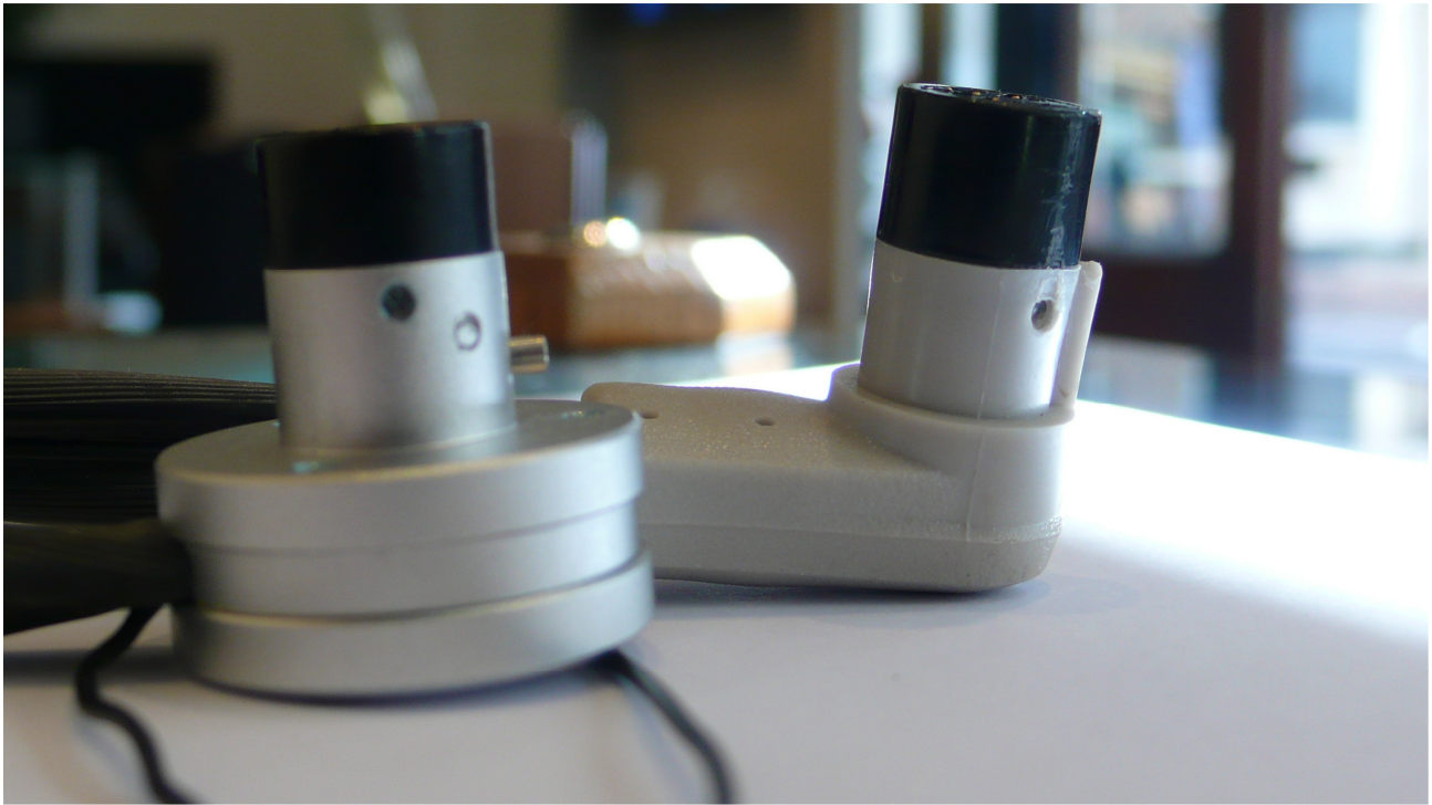
Figure 92 – Shows an old plastic plug (right) and an early metal plug (left) showing grub screw contact
