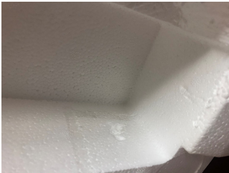
Figure 22 – indentations caused by cartridge and fingerlift
