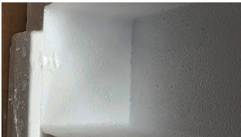
Figure 20 – dents in polystyrene caused by cartridge
