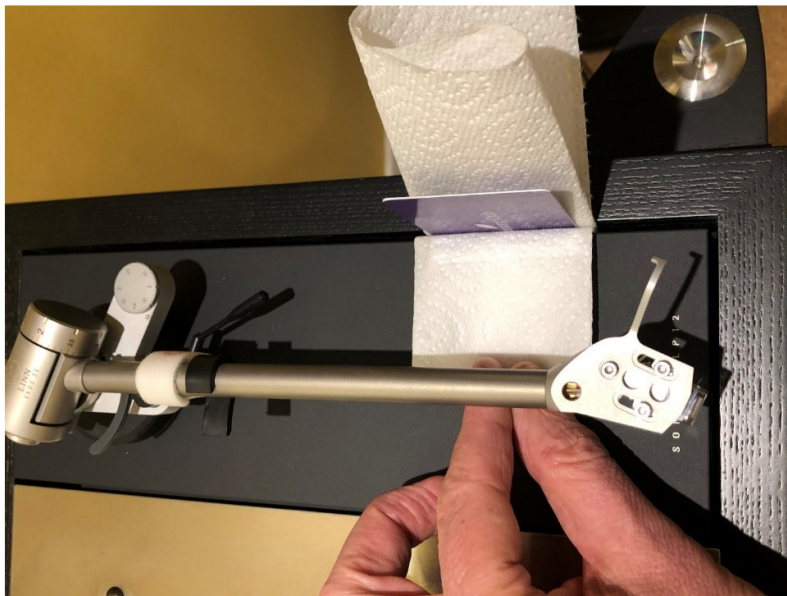
Figure 7 – using a credit card to insert the kitchen paper towel
