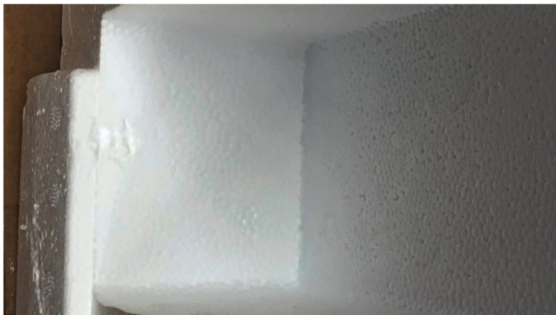
Figure 20 – dents in polystyrene caused by cartridge
