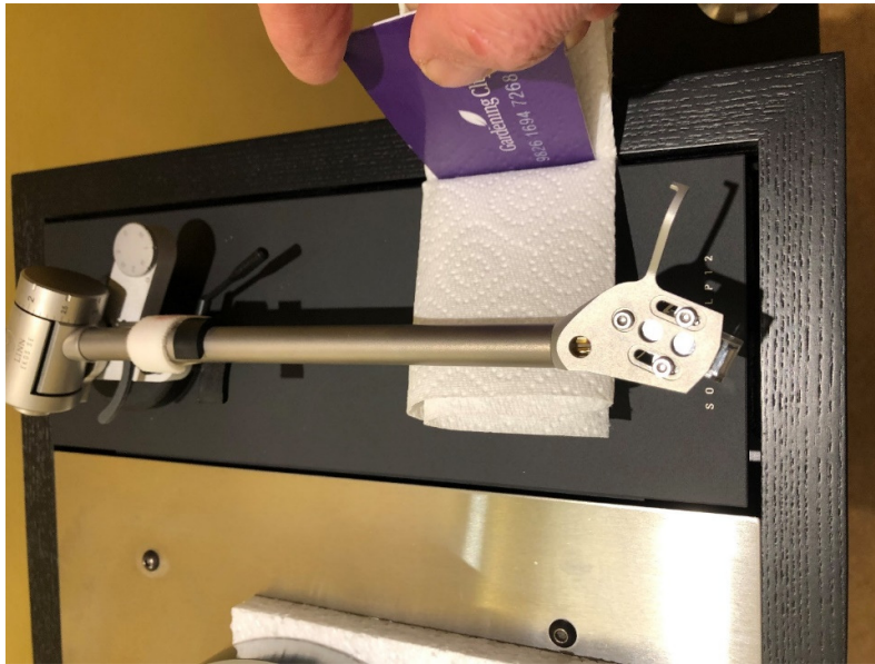
Figure 6 – limiting suspension movement
