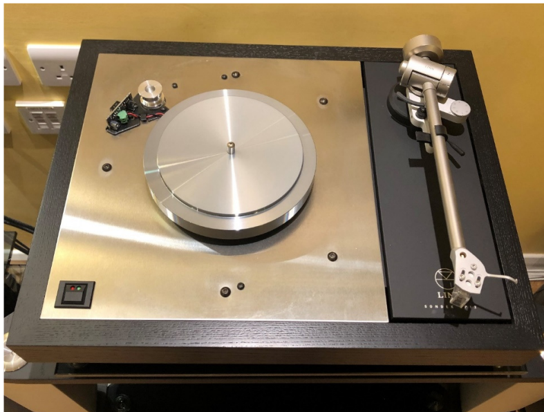
Figure 1 – outer platter removed and stylus guard fitted
