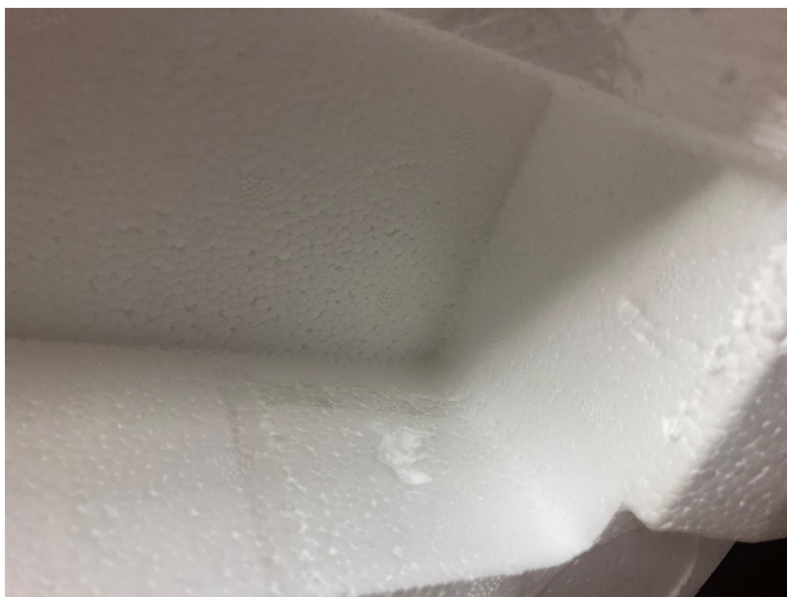
Figure 22 – indentations caused by cartridge and fingerlift
